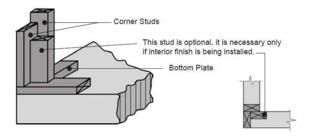
Figure 7 — Exterior Wall Framing at Gable End  $\,$  Detail
